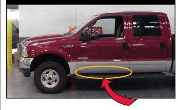
With a basin positioned below the fuel/water drain plug, remove fuel/water drain plug and drain until fuel stops.
