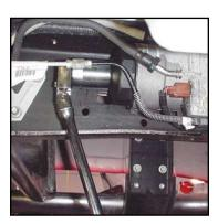
Re-attach the water and fuel drain plug. This completes the primary fuel filter change.
