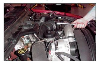
Remove fuel filter and 0-ring.Caution: Fuel filter housing is filled with fuel.
