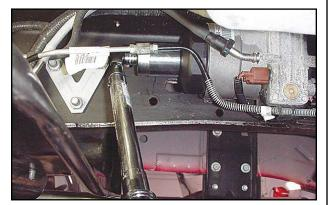
3. Remove primary fuel filter and O-ring from the end cap.
