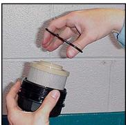
Screw the fuel end cap, with new filter and O-ring, back into housing. Torque to 25 Nm (19 lbs./ft.).
