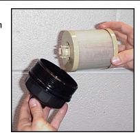
4a. Replace the primary fuel filter (large size filter in kit) by snapping a new filter element into the fuel filter end cap.
