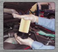
attached filter back into its housing and torque to 25Nm or 19lbf/ft, again using the 36mm socket and ratchet.
