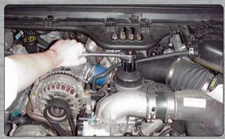
NOTE: Unscrewing the cap opens the oil filter drain and drains the oil from the oil filter housing into the crankcase.
