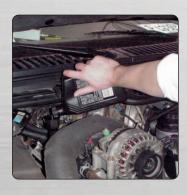
Start and run the engine for a few minutes, then stop the engine, open the hood and look for leaks.
