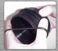
Insert the new oil filter element to the inside of the oil filter cap
