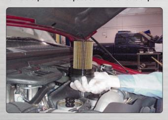
Using oil resistant gloves, detach the oil filter and O-ring from the re-usable cap and dispose of properly.
