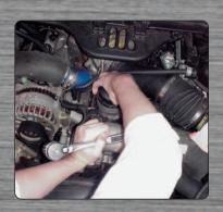
Warning: Tightening beyond torque specs will crack reusable oil filter cap.
